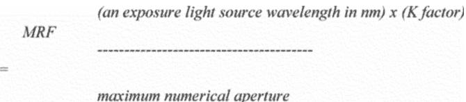
where, for the purposes of 3B001.f.1.b, the K factor = 0.25 'MRF' is also known as resolution. 2. 'Dedicated chuck overlay' is the alignment accuracy of a new pattern to an existing pattern printed on a wafer by the same lithographic system. 'Dedicated chuck overlay' is also known as single machine overlay.
