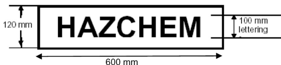
**Figure 13.1 Form and dimensions of outer warning placard**
